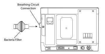
Installing a New Bacteria Filter
